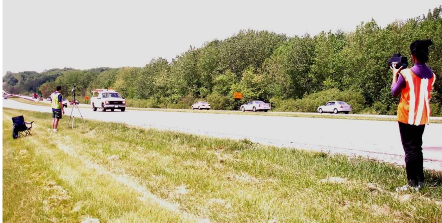
Figure 3.2. Measuring Vehicle Speed during SPB Measurement
