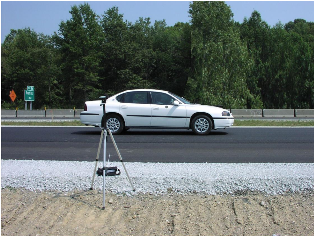
Figure 3.1. Pass-By Measurement Site (I74) and Microphone Setup
